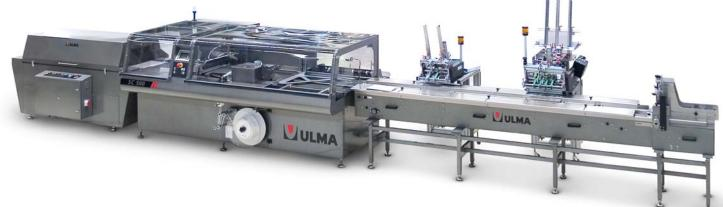
The automatic SC 500 continuous side seal machine has been designed to pack a great range of products whatever might be the length, with shrink and non shrink films, achieving productions up to 125 cycles/min.
